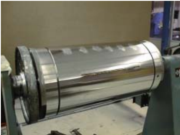
Fig. 4. The prototype bobbin wrapped with the 301 high yield stainless steel after welding.
