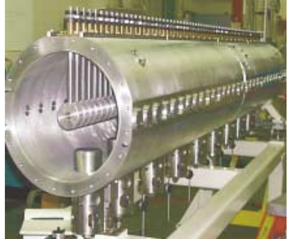
Figure 1. Full-scale aluminum model of DTL tank 1.
