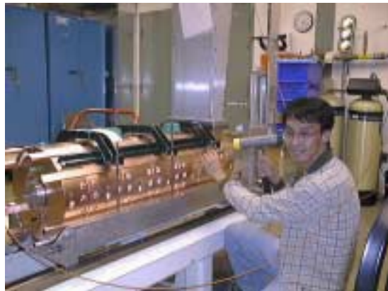
Figure 2: Open cell 805-MHz cavity at FNAL being tuned to final operating frequency in preparation for high-power testing.
