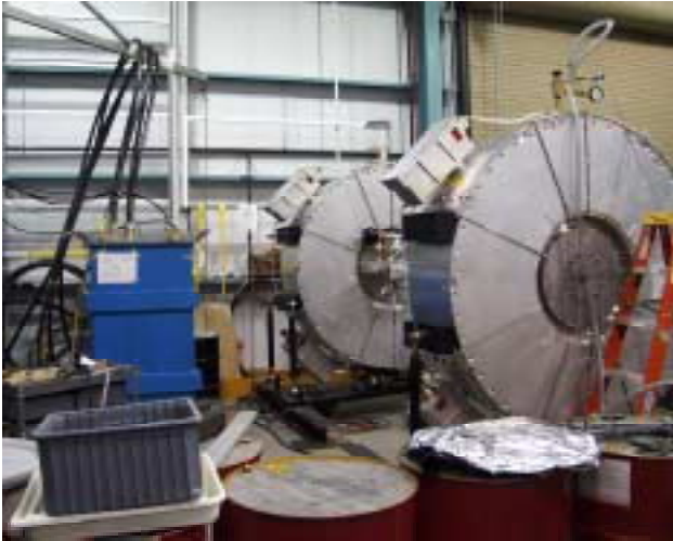
Figure 4: Induction linac cores fabricated at LBNL for the DARHT project; these are representative of the cores that would be used in a Neutrino Factory.
