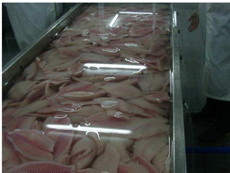
**Figure 3** – Tilapia fillets washing with ozonized water.
