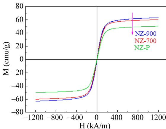
**Figure 5.** Magnetic hysteresis loops of specimens NZ-P, NZ-700 and NZ-900 at room temperature.
