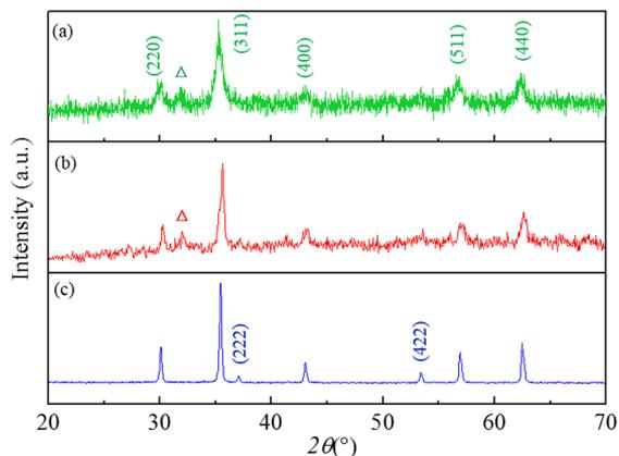
**Figure 1.** XRD patterns of specimens NZ-P (a), NZ-700 (b) and NZ-900 (c). The marked peak disappeared in (c). A special peak marked by “ $\Delta$ ” from specimen in (a) and (b) disappears in (c).
