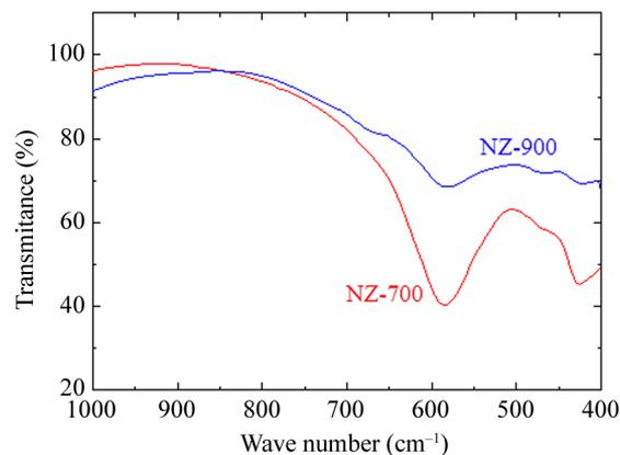
**Figure 4.** FTIR spectra of specimens NZ-700 and NZ-900.
