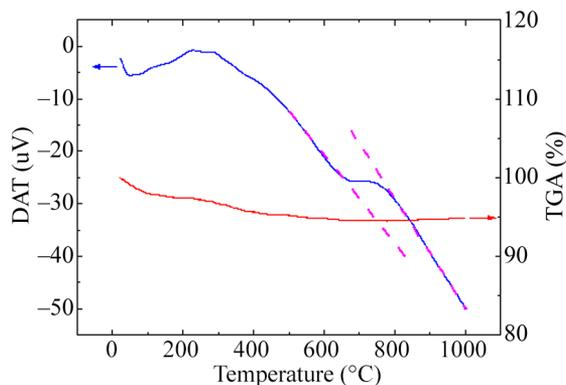
**Figure 3.** TGA-DTA curves of specimen NZ-P. The dash lines are guide for eyes.
