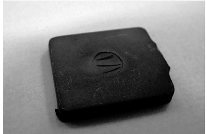
**Figure 4.** Coloured surface suggesting evaporation of copper during sintering at 1 mbar.
