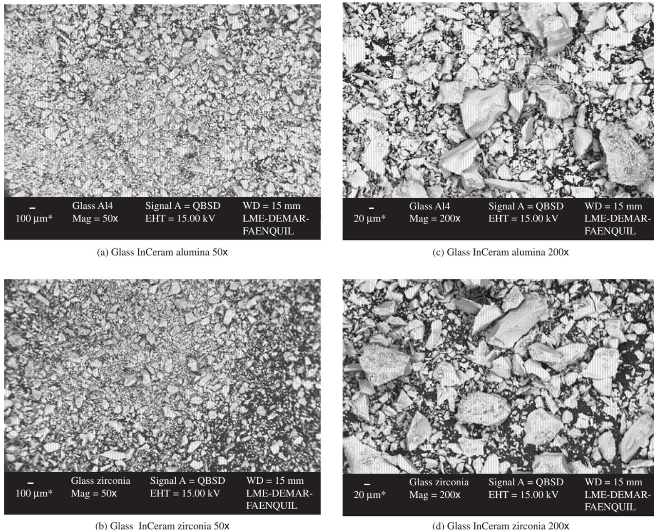
**Figure 3.** SEM micrographs of the InCeram glass powders: a,c) InCeram alumina; and b,d) InCeram zirconia.
