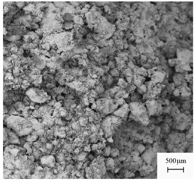
**Figure 10.** SEM micrograph of a general view of the (J) samples (CPI-S-32 cement/5% bottom ash/sand) after 28 days of aging.
