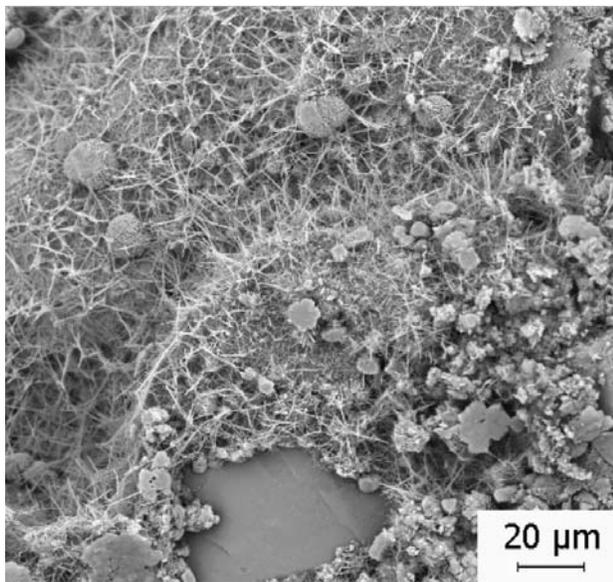
**Figure 9.** SEM micrograph of the anhydrite crystals in sample (K) (CPII-Z-32 cement/10% bottom ash/sand) after 28 days of aging.
