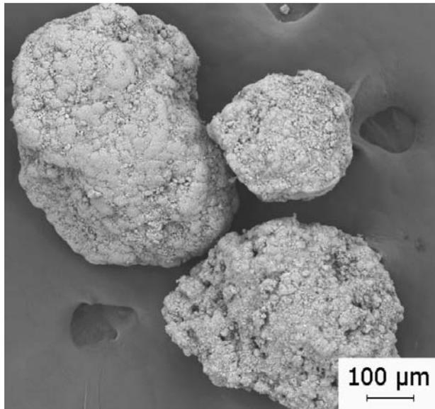
**Figure 4.** SEM micrograph of the morphology of the as received grit.
