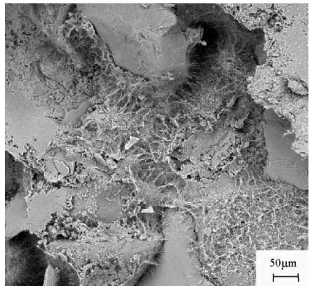
**Figure 7.** SEM micrograph showing gel crystallization on the (Rs) Matrix (CPI-S-32 cement/sand) after 28 days of aging.
