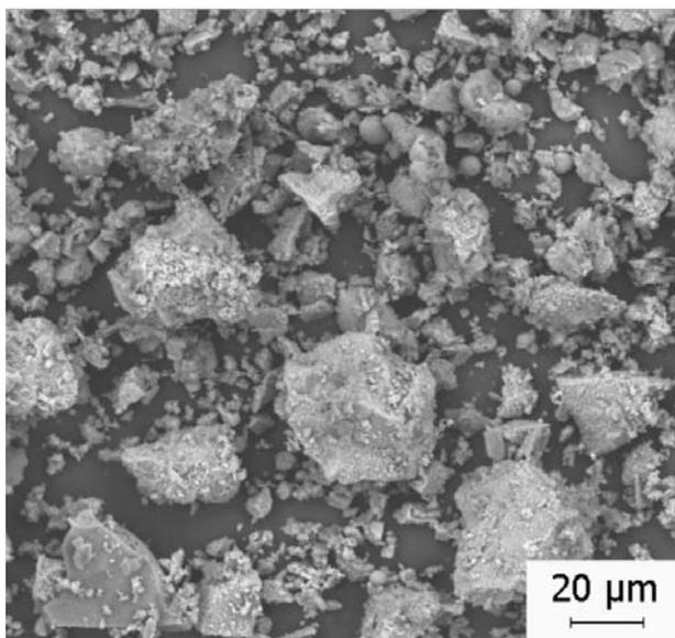
**Figure 1.** SEM micrograph showing the morphology and impurities, mainly inert ash, in CPII-Z 32 Portland cement powder.
