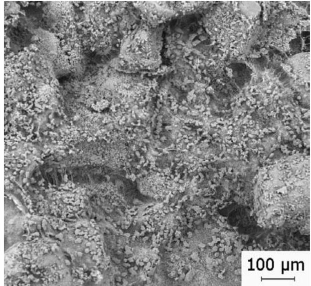
**Figure 14.** SEM micrograph of the aggregate/gel interface in the (L) samples (CPII-Z-32 cement/sand/5% grit) after 28 days of aging.
