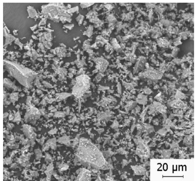
**Figure 3.** SEM micrograph of the morphology of bottom ash waste powder.
