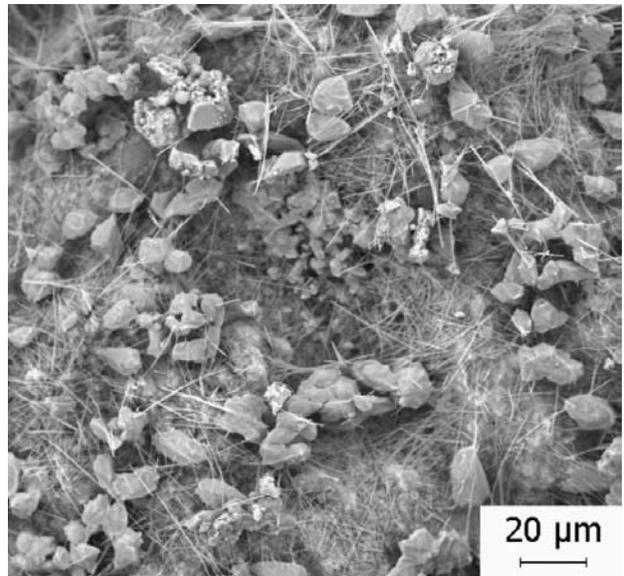
**Figure 15.** SEM micrograph of anhydrate crystals on the (L) samples (CPII-Z-32 cement/sand/5% grit) after 28 days of aging.
