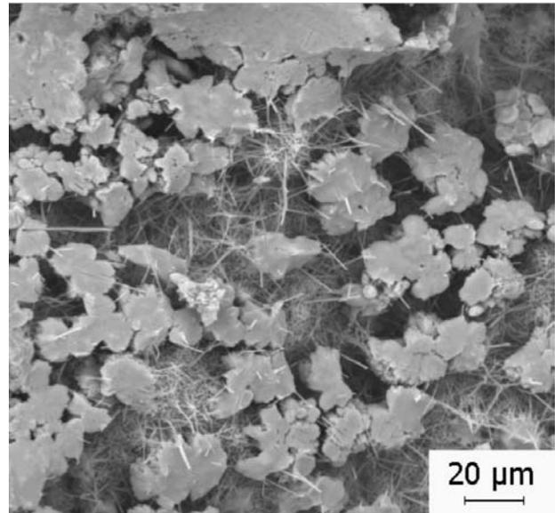
**Figure 6.** SEM micrograph of the porosity and disordered development of anhydrite crystals on the (Rz) Matrix (CPII-Z-32 cement/sand) after 28 days of aging.
