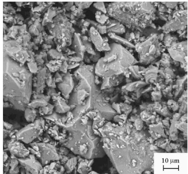
**Figure 2.** SEM micrograph of the morphology of CPI-S-32 Portland cement powder.
