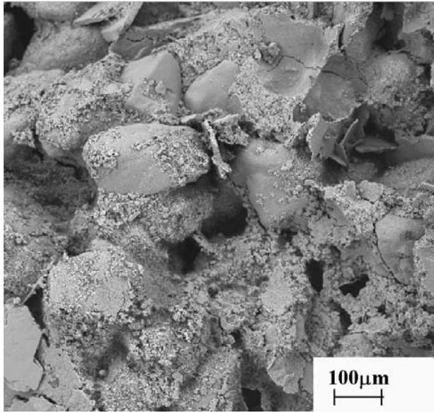
**Figure 8.** SEM micrograph of the porosity and aggregate/gel interface of sample (K) (CPII-Z-32 cement/10% bottom ash/sand) after 28 days of aging.
