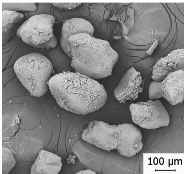
**Figure 5.** SEM micrograph of clay coating the sand grains.
