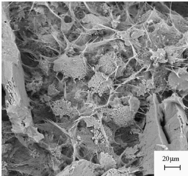
**Figure 13.** SEM micrograph of the aggregate/paste interface in the (J) samples (CPI-S-32 cement/5% bottom ash/sand) after 28 days of aging.
