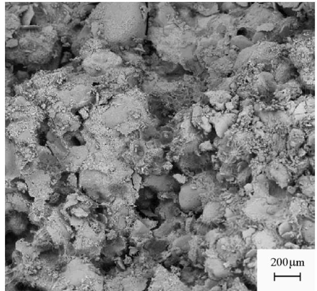
**Figure 11.** SEM micrograph of the aggregate partially covered by bottom ash powder in the (J) samples (CPI-S-32 cement/5% bottom ash/sand) after 28 days of aging.
