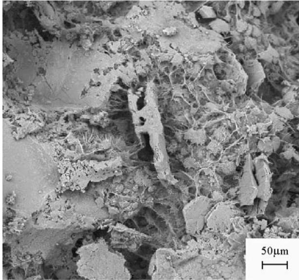
**Figure 12.** SEM micrograph of crystals growing on the surface of aggregates in the (J) samples (CPI-S-32 cement/5% bottom ash/sand) after 28 days of aging.
