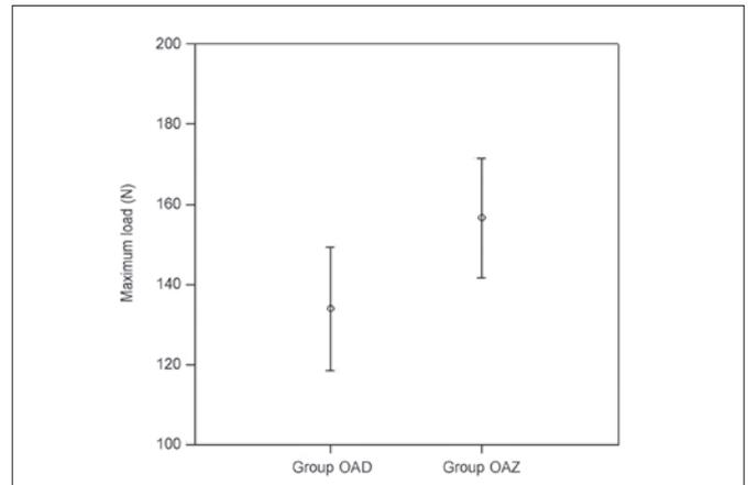
**Figure 10** – Mean maximum load at the time of the fracture in groups OAD and OAZ ( $p=0.005$ ).
