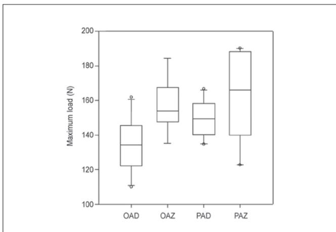
**Figure 9** – Box plot of the median of maximum load at the time of the fracture in the different groups ( $p=0.02$ ).
