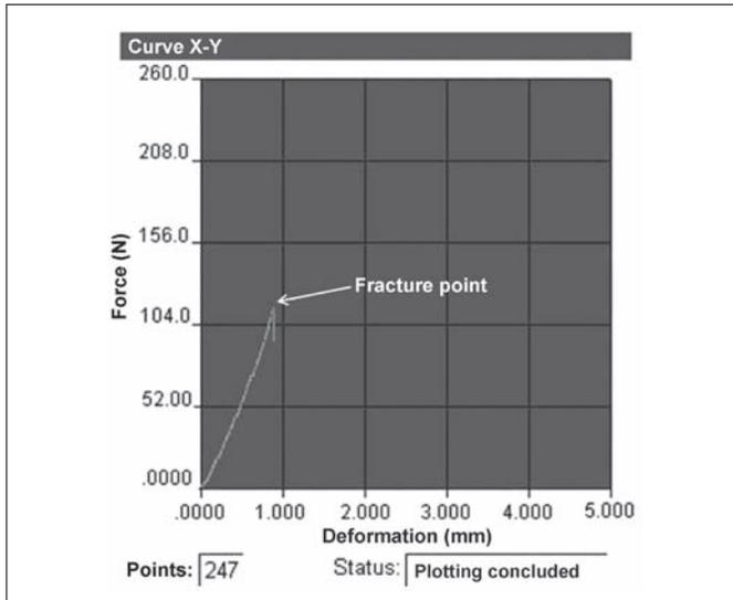
**Figure 3** – Load-deformation diagram obtained during the axial compression assay.
