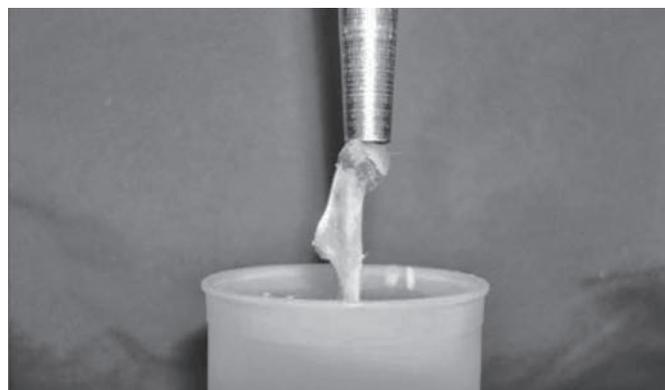
**Figure 2** – Detail of the test specimen at rest and of the load application bone cleaver, positioned axially to the humeral head.
