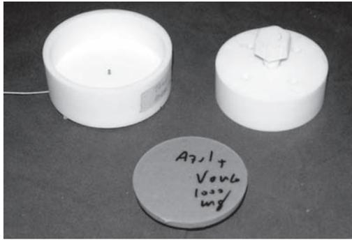
**Figure 7** – Thermocouple inserted on the cast base and cement removed after the assay in order to determine the maximum temperature.
