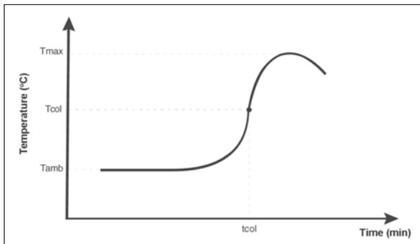
**Figure 8** – Typical curve for determining maximum temperature and insertion time.
