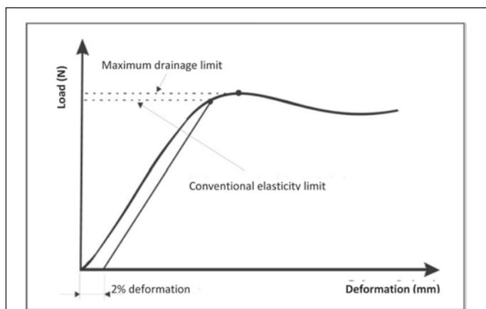
Figure 4 – Typical curve for load versus deformation in a cement compression assay
