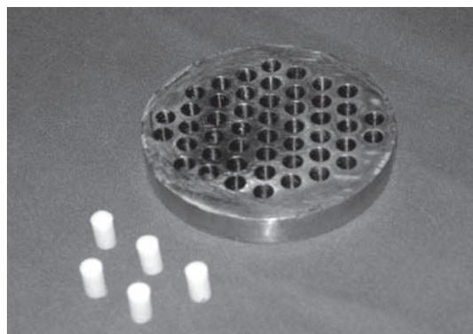
**Figure 3** – Cast and cement cylinders used on the compression assay
