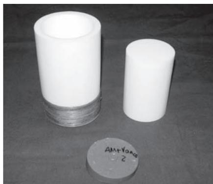
**Figure 2** – Cast, plunger and hardened cement used on the intrusion assay.
