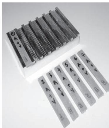
Figure 5 – Cast and bodies of evidence used on the cement folding assay
