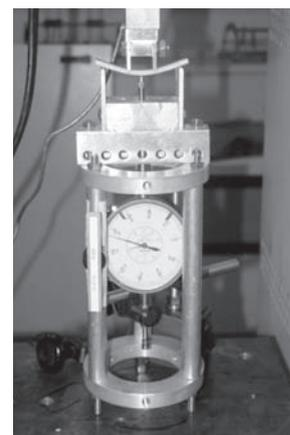
Figure 6 – Assay device for folding at four points and comparator clock
