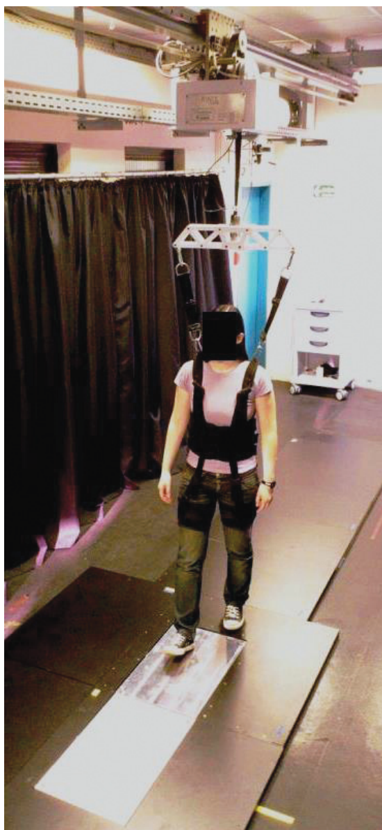
Figure 1. Partial view of the body weight support system employed in the present study and the walkway with built-in force plates. Note: during the experimental session, a thin rubber carpet covered the entire walkway.
