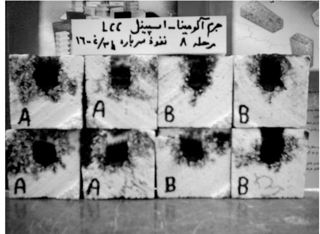
Figure 13: Slag penetration test alumina-spinel castable including (A= 2.5, B=3 %wt. microsilica).
