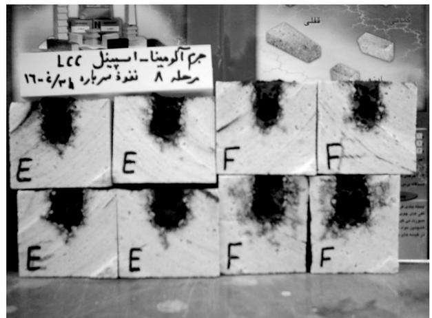
Figure 15: Slag penetration test alumina-spinel castable including (E= 4.5, F= 5 %wt. microsilica).
