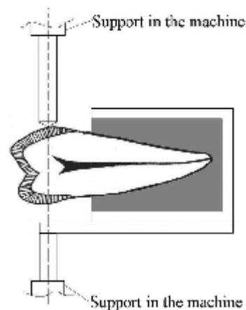
Figure 2. Schematic drawing of the customized flexural strength testing device.
