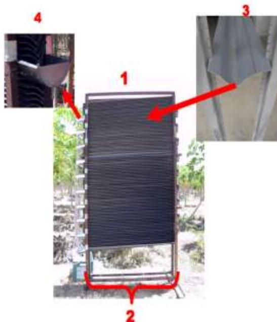
FIGURE 1. Front view of the vertical patternator (1- vertical patternator, 2- iron structure, 3- plastic gutters, 4- zinc funnel).
