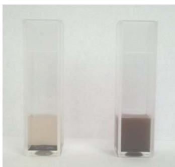
Figure 4. Bare (left suspension) and silanized (right suspension) images of CoFe 2 O 4 nanoparticles (0.02 mg/mL, pH 4). The instability of bare nanoparticles is clearly evident.
