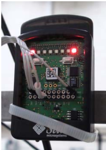
Figure 6. Detail of the serial RS232–USART interface.
