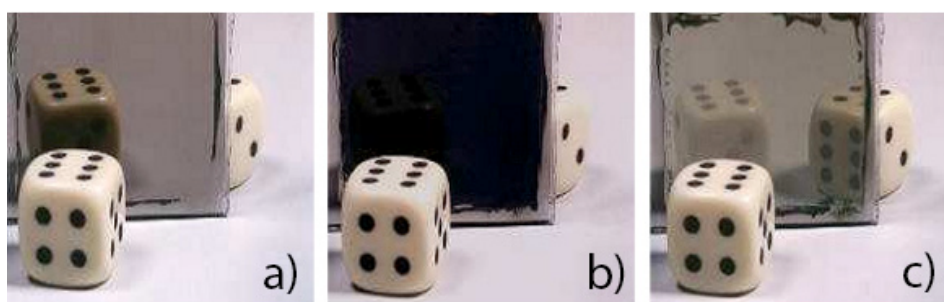
Figure 7. Three optical states of Mg-Gd switchable mirror: reflecting (a), absorbing (b) and transmitting (c) states [19].
