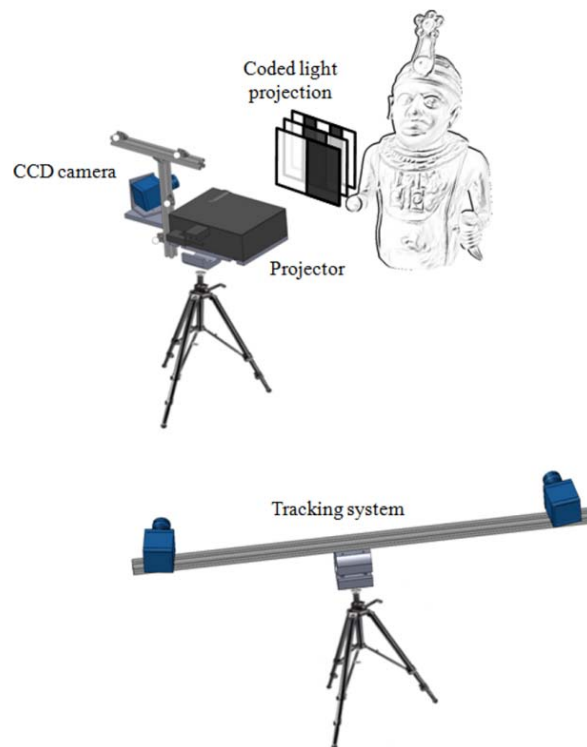
Figure 2. Scheme of the measurement process for a 3D artwork reconstruction.
