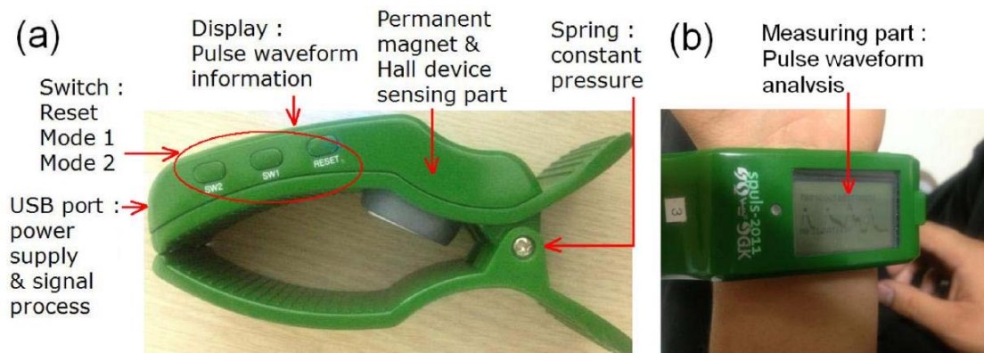
Figure 1. (a) The notation and function of several major parts and (b) the measurement process of acquisition pulse signals by a real clip-type pulsimeter.
