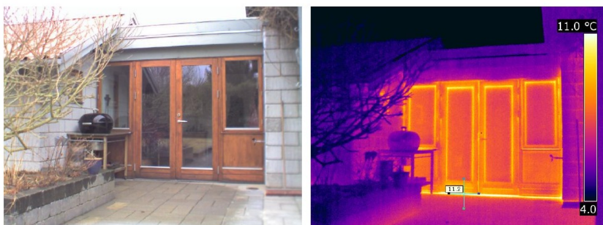
Figure 3. Poorly insulated window/door section along a corridor that connects the main house with an annex.
