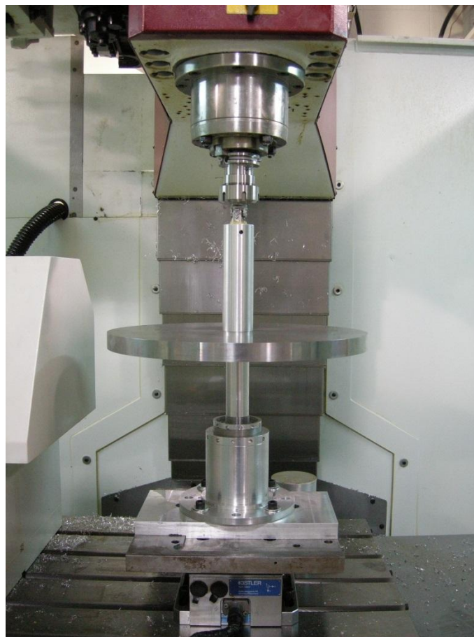
Figure 15. Experimental apparatus including the steel disk used to measure the damping.
