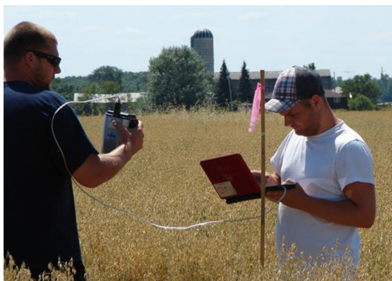
Figure 4. Preparing the ASD Inc. FieldSpec HandHeld Visible/Near Infrared portable spectroradiometer for measurements in an oat ( Avena sativa ) field in West Nipissing, Ontario, Canada.
