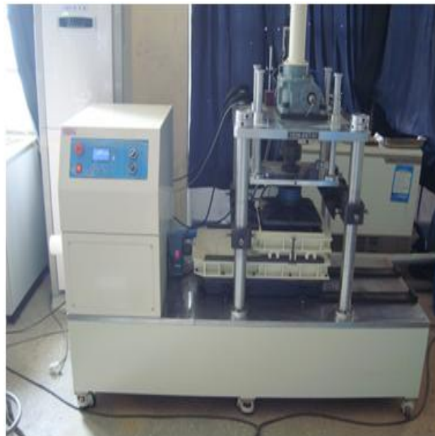
Figure 3. Large direct shear tester.
