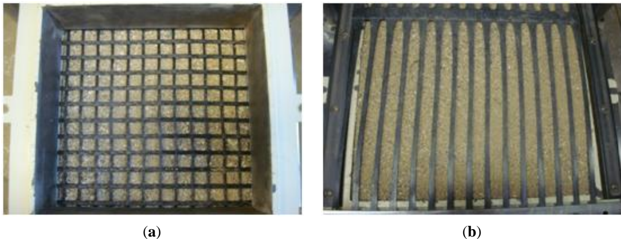
Figure 4. Geogrid was installed in the shear box: (a) Soft geogrid; (b) Stiff geogrid.
