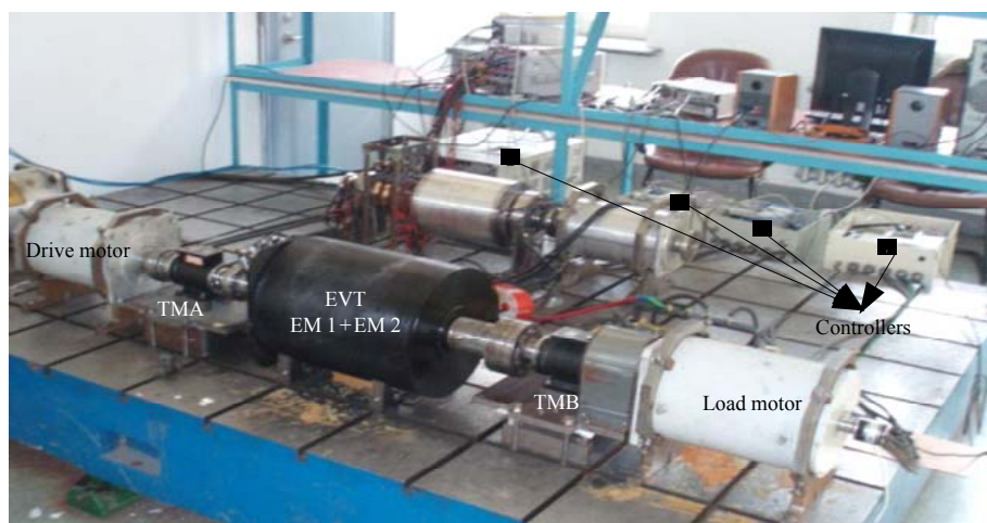
Figure 24. The EVT-based HEV experimental test bench.
