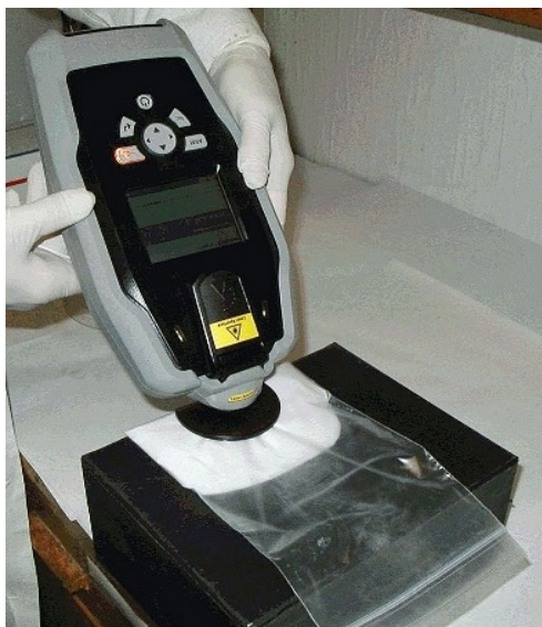
Figure 4. Portable Raman spectrometer FirstDefender.
