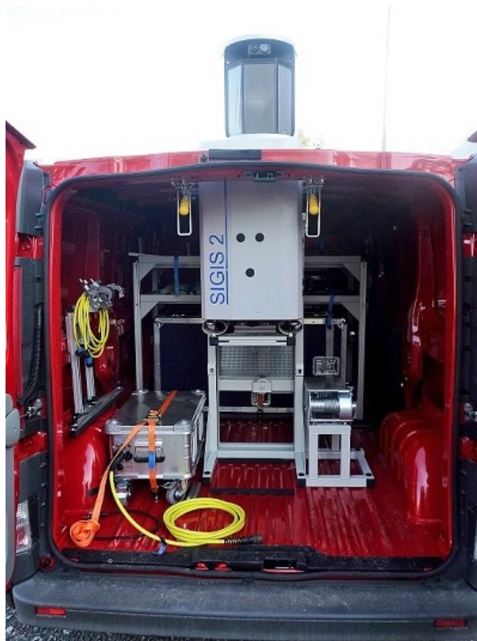
Figure 3. Monitoring vehicle with remote detector SIGIS 2.
