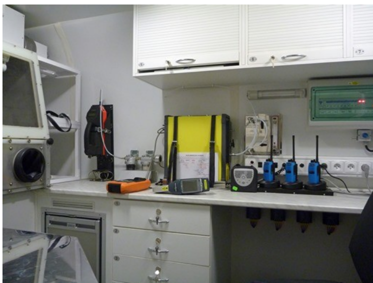
Figure 5. Laboratory section of the mobile chemical laboratory of the Fire and Rescue Service of the Czech Republic (FRS CR).
