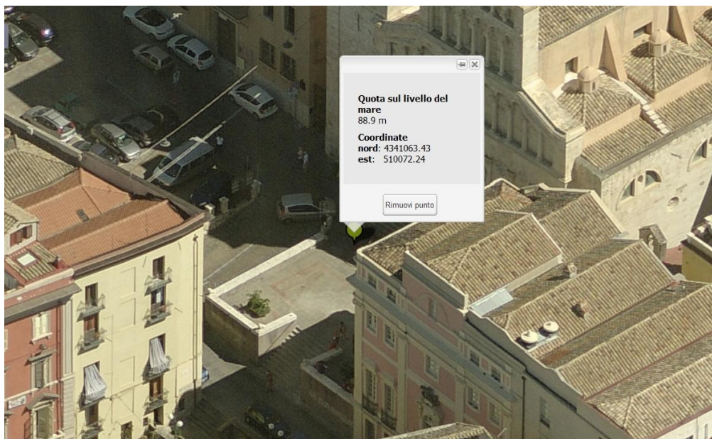
Figure 13. The algorithm precision is related to the DSM model being discrete. Thus, selecting the corner of a building might result in the algorithm calculating the elevation of the point that lies beyond the building itself.
