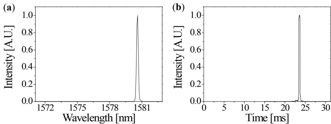
**Figure 6.** The static strain response of FBG in (a) the wavelength domain, and (b) the time domain.
