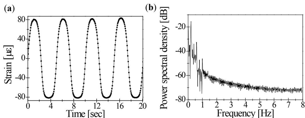
Figure 7a shows the corresponding output signals obtained by peak value of the FBG sensor interrogation system. The reflected FBG signals collected by the photodetector were effectively digitized by a data acquisition board at 10 MS/s. A total of 6400 samples were processed during 0.065 s for each single sweep of 16 Hz. The appropriate power spectral density (PSD) with a fast Fourier transform (FFT) spectrum was also measured for the dynamic strain, as shown in Figure 7b.
