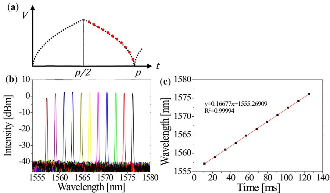
**Figure 3.** (a) OSA peak hold mode spectra of the linearized wavelength-swept thermo-optic laser output; (b) Time domain tracing of the laser output at swept rate ( $f_s$ ) of 16 Hz.
