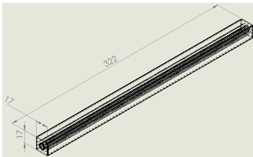
Figure 11. Dimensioned assembly drawing of the CFD study model.
