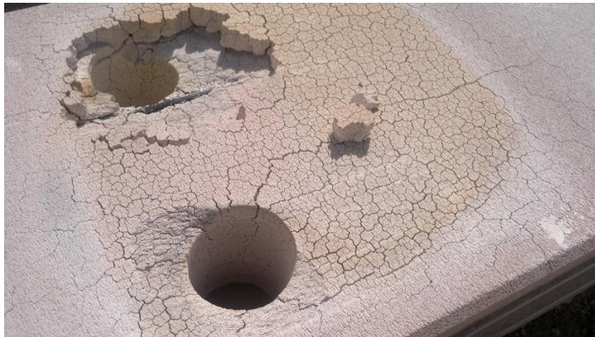
Figure 6. Autoclaved concrete (AAC) cracking and heat damage.
