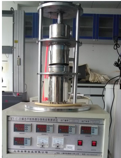
Figure 8. Schematic diagram of the thermal conductivity test.
