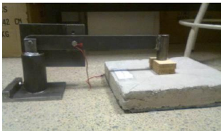
Figure 2. Hammer placed and levelled on wood blocks.
