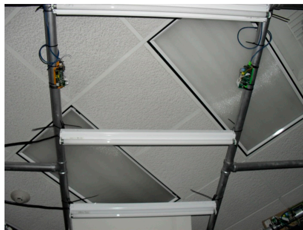
Figure 2. Cameras mounted on top of the scanner and the lighting configuration.
