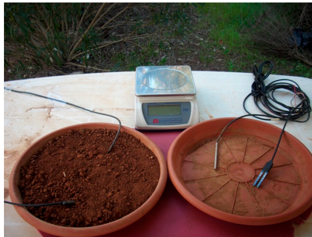
Figure 3. The two plates experimental arrangement. The plates are 35 cm in diameter and 4 cm in depth and are placed on an insulating sheet. The inserted sensors (thermometer Campbell 107L and soil moisture sensor Decagon EC-5) are also shown, together with the precision balance.
