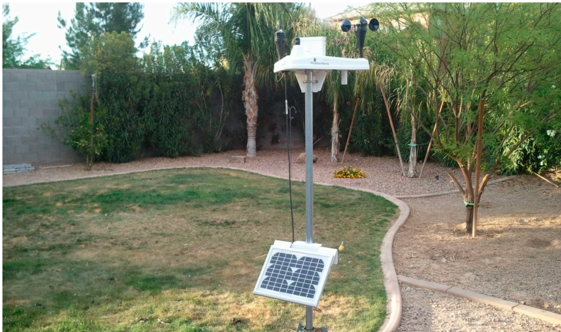
Figure 3. Micrometeorological towers used to monitor variables related to people's perceptions of their immediate climate. Towers include sensors that measure air temperature, relative humidity, wind speed, and light at 2 m height, as well as soil temperature, soil moisture, and irrigation water use (photo credit, B. Ruddell).
