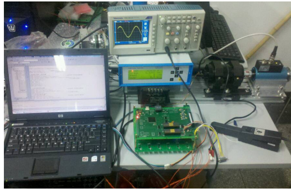
Figure 12. Test bench for measuring torque at load.
