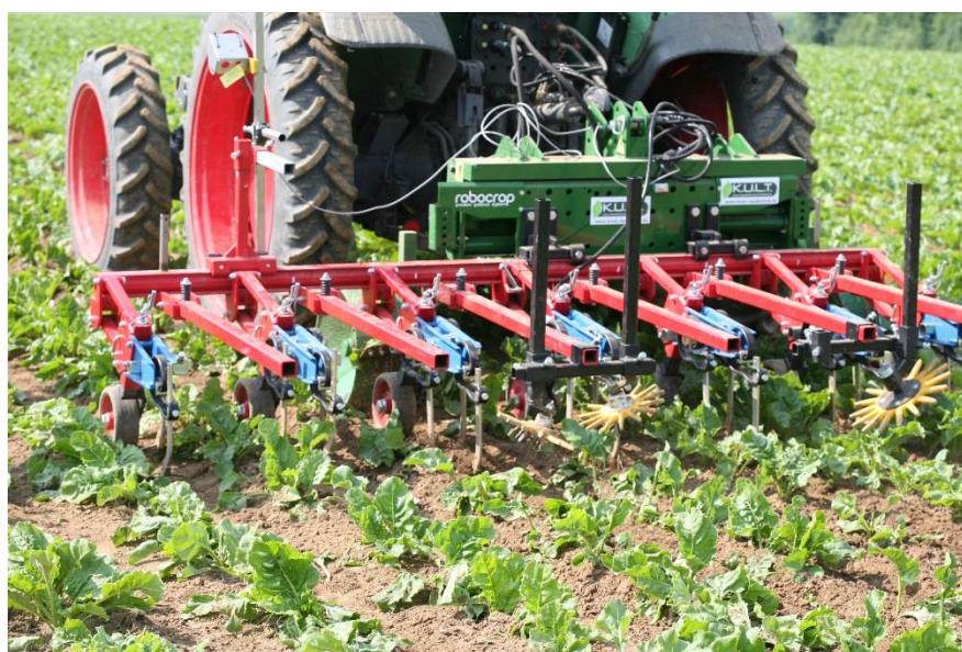
Figure 4. Photo of the Kult-robocrop ® hoe with a camera-based automatic steering system in sugar beet at 8-leaf stage at Ihinger Hof.
