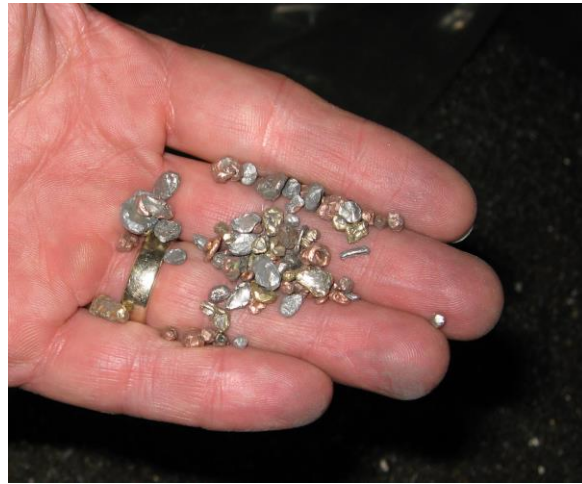
Figure 4. Example of shredded particles of an old computers (this illustrates the end product of re-manufactured old computers).
