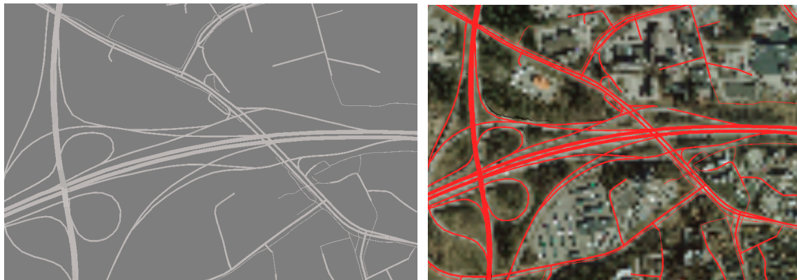
Figure 26. The result of 3D road network reconstruction. (Left) 3D road networks; (Right) 3D roads overlaid on the NLS orthophoto (roads in red).
