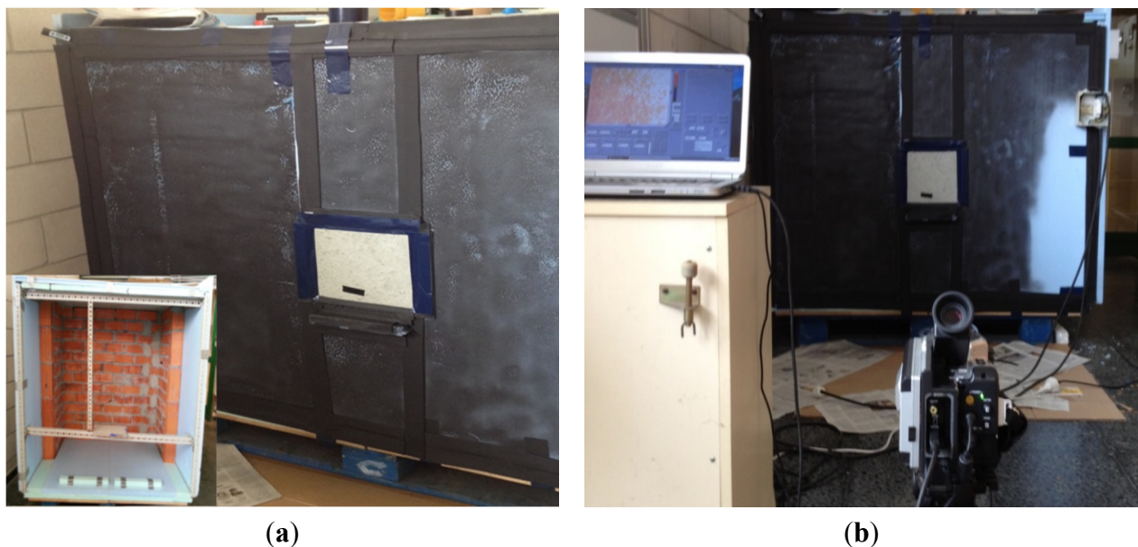
Figure 1. (a) Cabin painted black with specimen centered. Bottom left: cabin without the front panel, with support area for the specimen; (b) Measuring and recording equipment.
