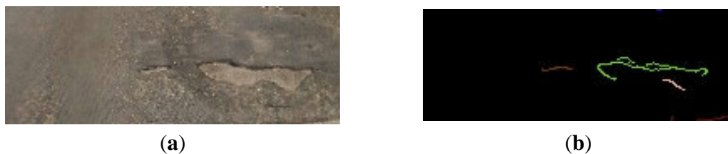
Figure 7. (a) Pothole on the road (b) corresponding edge information.
