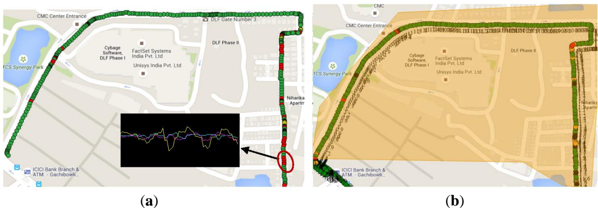
Figure 17. Results comparison for moderately rough road. (a) is the Road Condition Results Map from MAARGHA (sub image: accelerometer readings), while (b) is from Roadroid (Screenshot from its cloud server).
