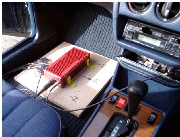
Figure 10. Measurement of the hybrid electric vehicle with RT3102.
