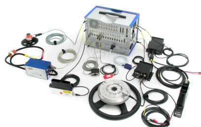
Figure 5. Connections for the Dewetron testing system.
