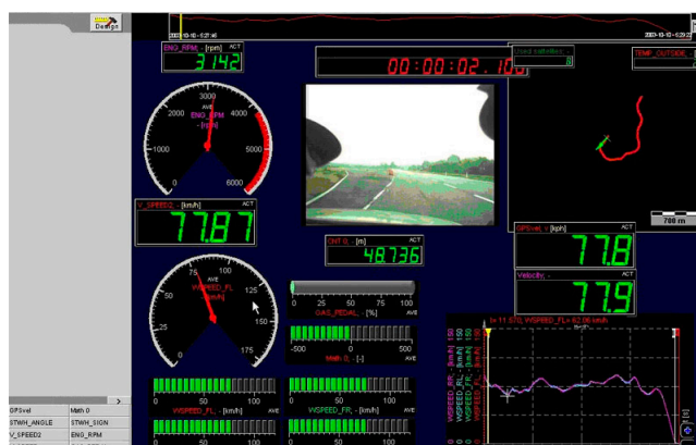
Figure 4. Graphical interface of the Dewetron testing system.
