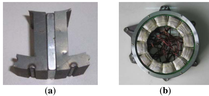
Figure 6. One module (a) and the assembly (b) of the stator.
