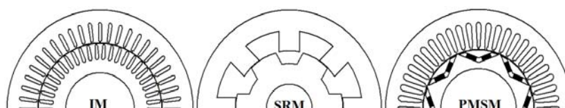
Figure 3. Three popular motors in EV: Induction machines (IM), switched reluctance machines (SRM) and permanent magnet synchronous machines (PMSM).
