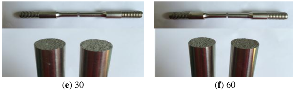
Figure 6. Comparison of fracture surface of SDSS tensile specimens according to various isothermal ageing periods (tested at 20 °C). (a) 0 min; (b) 5 min; (c) 10 min; (d) 15 min; (e) 30 min; (f) 60 min.
