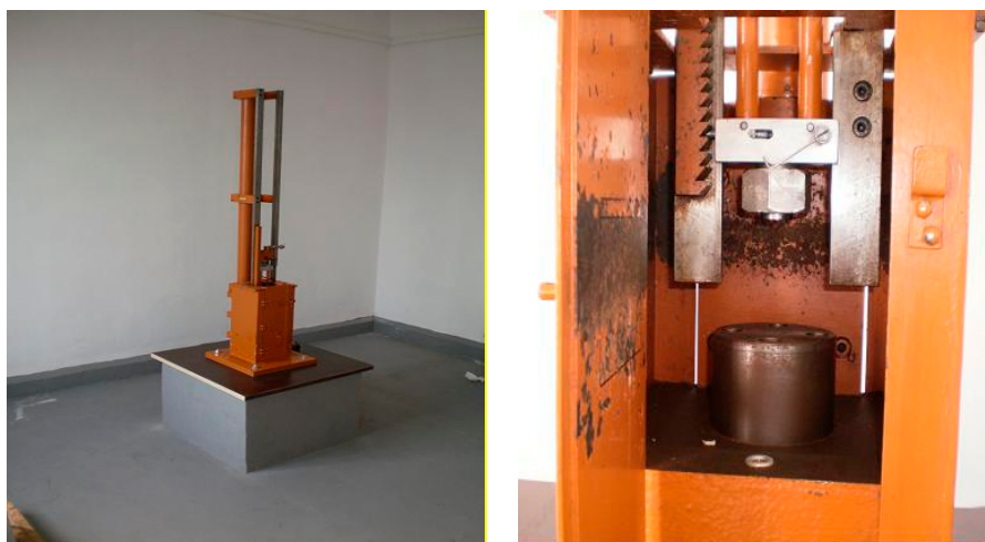
Figure 10. BAM drophammer setup used in this study.
