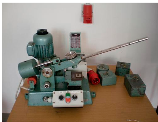
Figure 11. BAM friction test setup used in this study.
