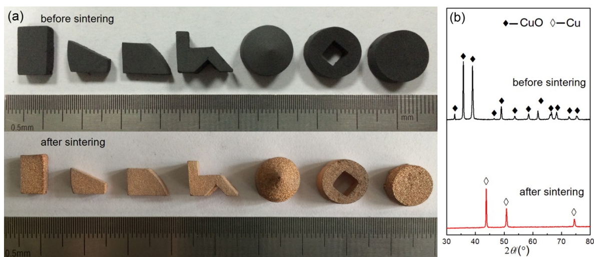
Figure 3. Macro photograph (a), and XRD patterns (b) of the porous bodies (30 vol.%) before and after vacuum sintering.
