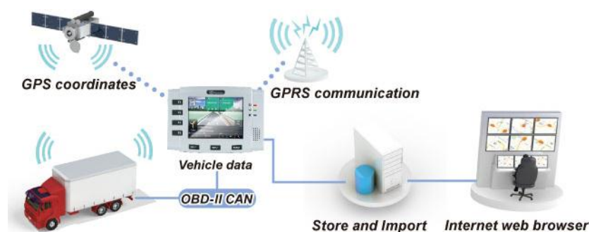
Figure 3. Truck management system architecture scheme [21]. GPS: global positioning systems; GPRS: general packet radio service.
