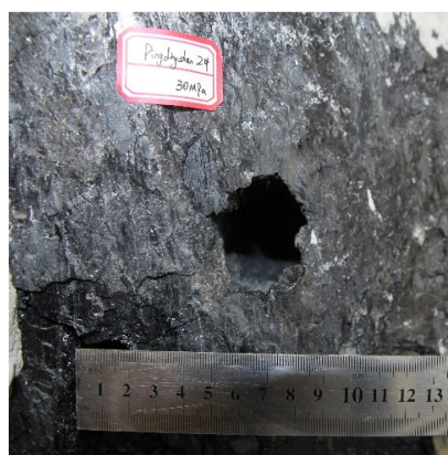
Figure 6. Coal sample from the Pingdingshan mine used for drilling tests.
