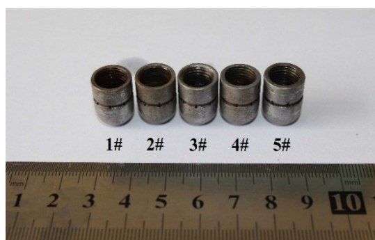
Figure 12. Self-propelled nozzles with different backward orifices axial angles.
