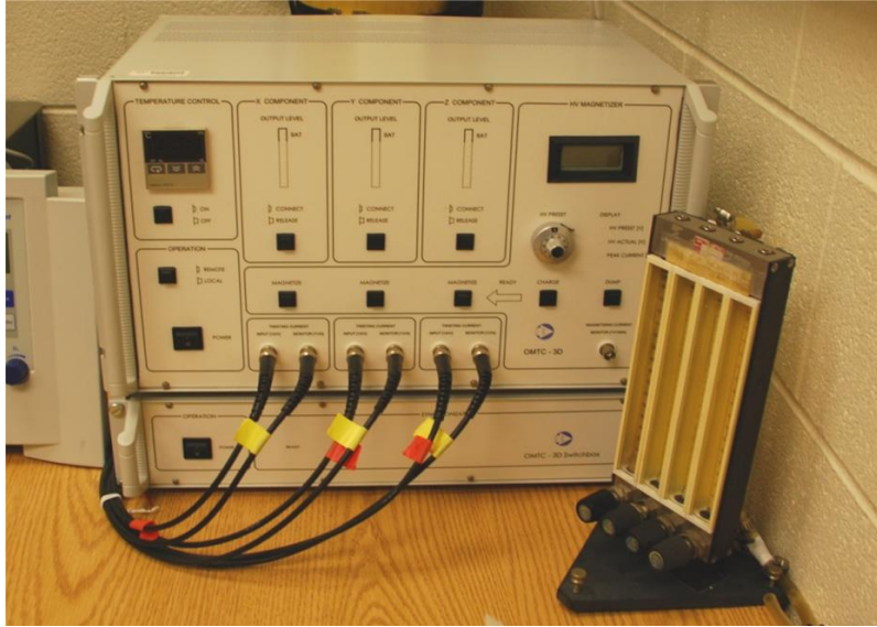
Figure 2. Image of the MTC control unit. This unit is linked to a computer where parameters such as magnetic field strength, oscillation frequency and waveform (sinusoidal or step function) are set. Once the parameters are set, the MTC control unit sends current to the MTC. Bead magnetization is done by pressing the charge button and then pressing a button corresponding to the desired orientation. The unit also controls the temperature of air running into the MTC.
