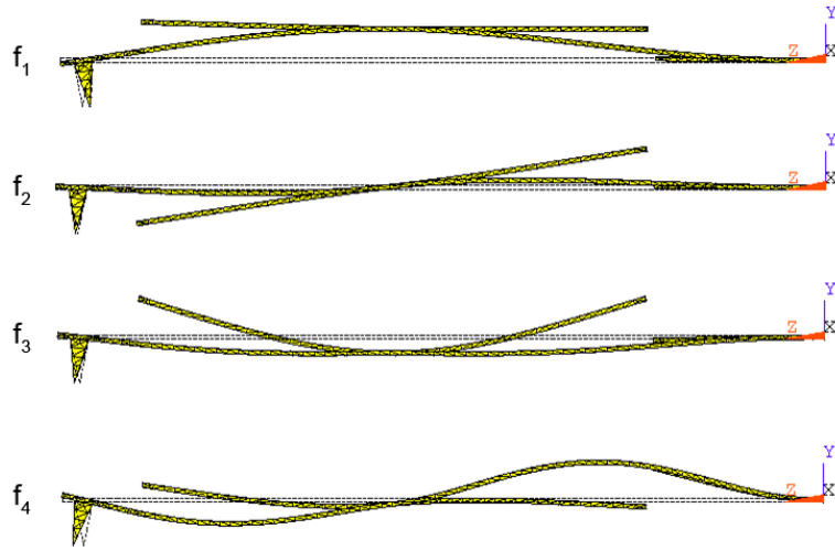
Figure 2: First four mode shapes for the internal torsion paddle cantilever fixed at the base and simply supported at the probe tip. The shape of the mode shows where high stress locations are, as well as providing insight into how the laser deflection system of the AFM will detect the probe response along the probe length.
