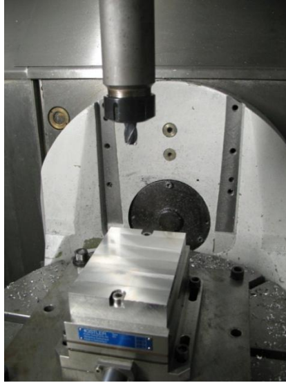
Figure 3.9: Tool and holder combination used in the experiments; the workpiece is mounted on the dynamometer. I would like to thank Raúl Zapata for allowing me to use this figure.
